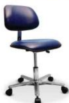
CLEANROOM TYPIST CHAIR - Material: Antistatic PVC Leather, chrome plated cylinder, polished aluminium chair base - Surface resistivity: 10e6 to 10e9 ohm/sq - Color: Blue & Black - Adjustable Height: Low: 390mm, High: 510mm
